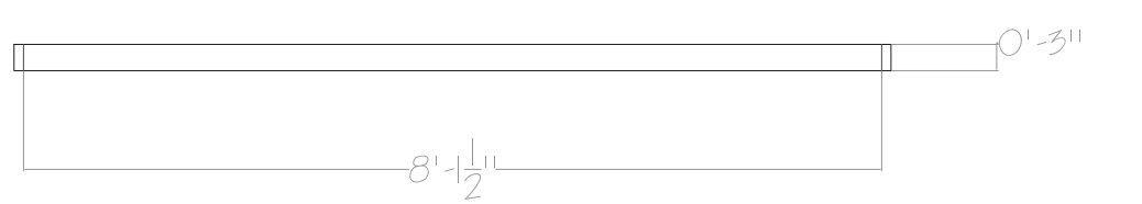
5 PLATFORM 'Q' FASCIA BOARD SCALE: 1/2" = 1'-0"
